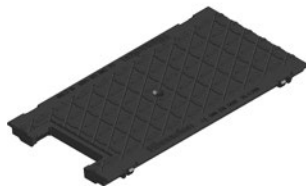
Ductile iron solid cover with opening for cables (128 mm x 49 mm), black, KTL, class C 250
